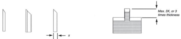
If x is the thickness of your knife NEVER grind a profile deeper than 3 X the knife thickness!
